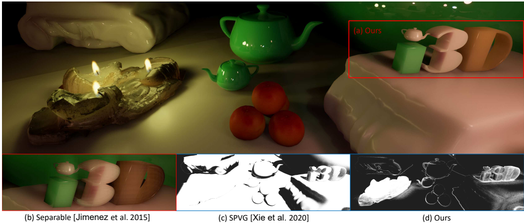
Fig. 1. Dynamic subsurface scene just after light has been turned off. Our method has consistently lower sample count (d) than SPVG [Xie et al. 2020] (c) at this frame. It leads to lower sampling pass time in dynamic lighting from 12.9 ms to 5.2 ms at 3360 \times 1440 ( \times 2.5 ), while maintaining good quality (47.5 dB) vs SPVG (48.6 dB). Separable (b) runs fastest for the whole subsurface pass at 4.0 ms, however, with visible banding artifacts.
