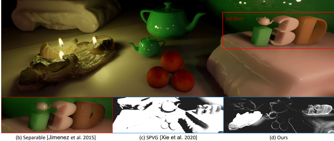
Figure 6.1: Dynamic subsurface scene just after light has been turned off. Our method has consistently lower sample count (d) than SPVG [Xie et al., 2020] (c) at this frame. It leads to lower sampling pass time in dynamic lighting from 12.9 ms to 5.2 ms at 3360 \times 1440 (\times 2.5) , while maintaining good quality (47.5 dB) vs SPVG (48.6 dB). Separable (b) runs fastest for the whole subsurface pass at 4.0 ms, however, with visible banding artifacts.
